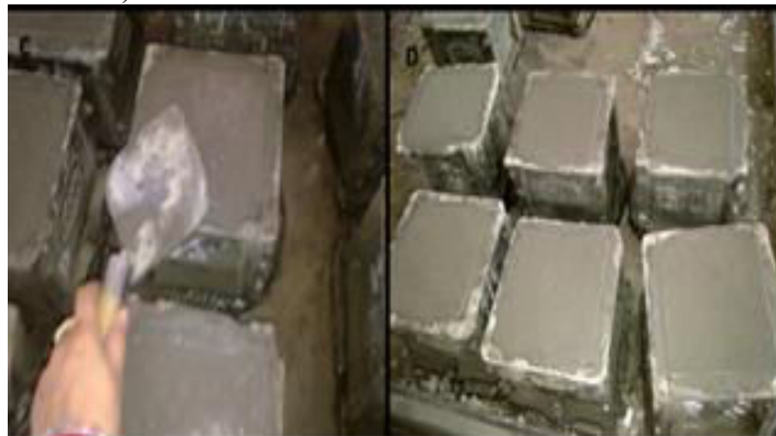
Fig. 2. Casting of Concrete Cubes (M20)
